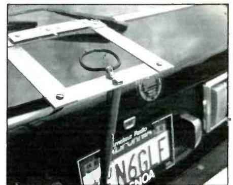
The VHF loop offers equal performance to longer mobile whips.
