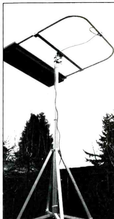
The small quad may be easily mounted by a tripod in an emergency.
